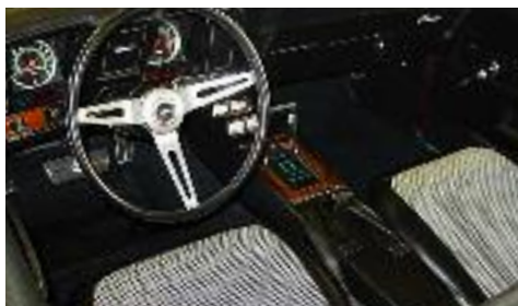
The '69 got square pods for the speedo and tach. This one has the desirable deluxe interior with houndstooth fabric and full console with gauges.
